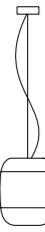
S3 Ceiling Rose Ø 120 mm Ceiling Rose LED Ø 160 mm Ceiling Rose LED DIMM Ø 200 mm Cable 2000 mm Diffuser Ø 300 mm H 375 mm
